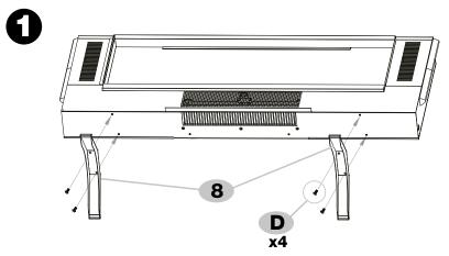
NOTE: Baffle 9 MUST be used for on feet installation
