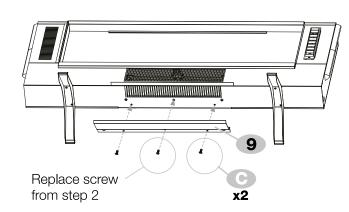
Baffle 9 MUST be used for "on feet installation"
